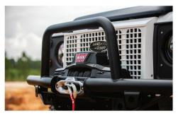
• Tubular winch bumper with 10s Platinum Warn wireless winch system
